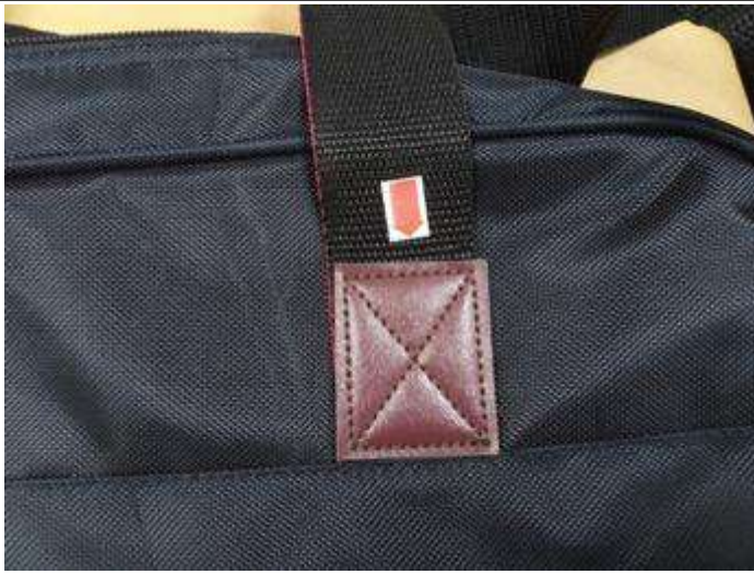
Poor stitches slightly
